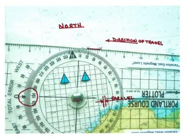
Reading the zero point on the plotter shows the vessels heading and in this example it is 278°
