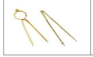
**Dividers** – set the dividers from the marked target position to the nearest printed line of latitude. Transfer the dividers to the scale at the side of the chart with one point on the chosen printed line of latitude and note the latitude reading shown by the other point of the dividers.
