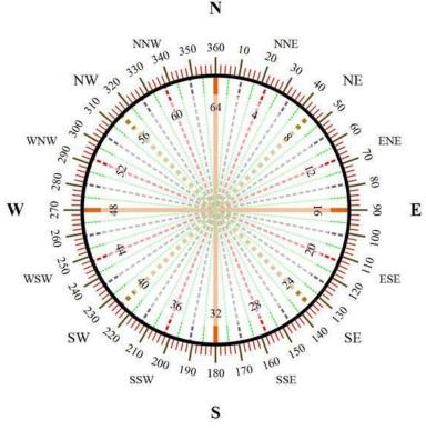
19. **Bearings** are measured clockwise from  $0^{\circ}$  (north) and are expressed in three figures, for example. 045° (north east), 090°(east), 270°(west).
