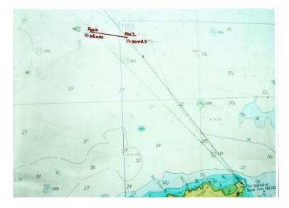
Next the Bretton Plotter is placed between these two positions and a line drawn between the two, the compass rose of th plotter is then turn to North.
