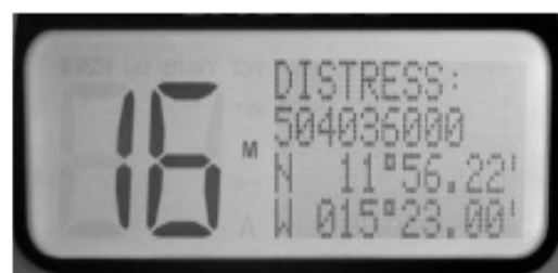
DSC radio Distress display showing casualty's MMSI and position
